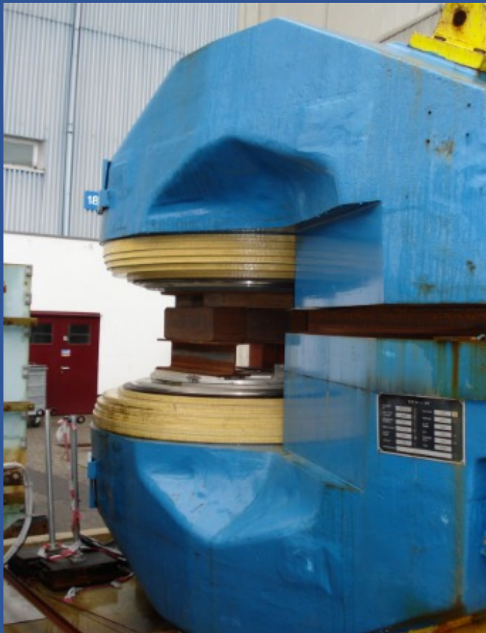
MEP48 dipole magnet Field 1.5 T over a 400mm gap
