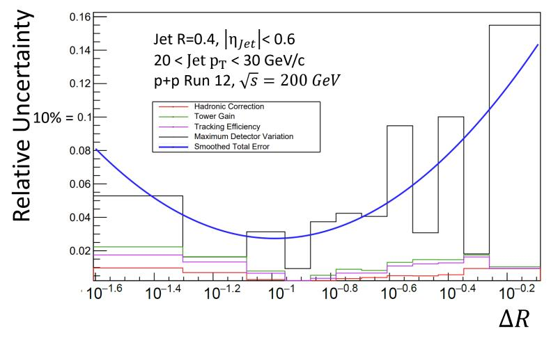
As shape correction needed is small, systematic uncertainties determined for the correction procedure are small.
